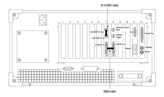
Figure 2–1: Cable connections on the MTS400 Series system
